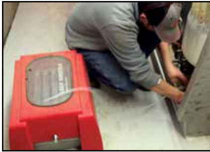
A piece of equipment called a shuttle is used to collect samples for monthly DHI tests for herds on official test, including Meier Dairy, the first herd to install robots in Kansas..
